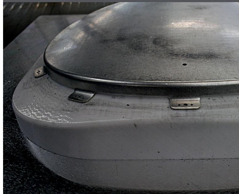
A formed aluminum window pan shown on top of the FDM hydroform tool.
